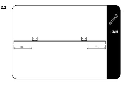
Looking from the side of the vehicle, position the Leg Mounts (Item 3) to center the Slimline II Rack or place Load Bars where desired over the load bed.
