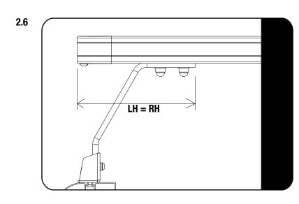
Conter the rack on the Legs before fully tightening (LH = RH).
