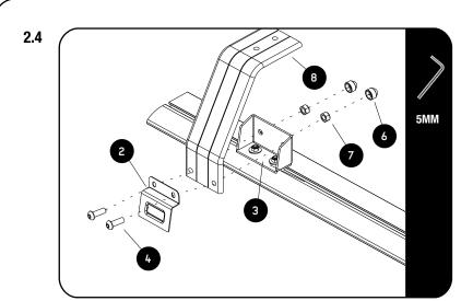
Assemble the Legs (Item 8) to the Leg Mount (Item 3) by using M8 x 30 Button Heads and M8 nyloc Nuts (Items 4 & 7) and the M8 x 20 T-Bolts (Items 1).
