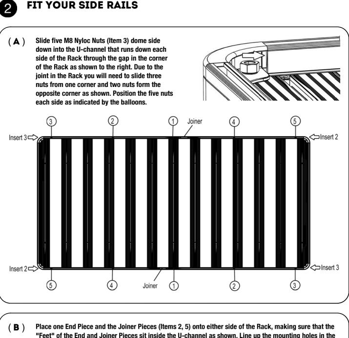
**B**) Place one End Piece and the Joiner Pieces (Items 2, 5) onto either side of the Rack, making sure that the "Feet" of the End and Joiner Pieces sit inside the U-channel as shown. Line up the mounting holes in the End and Joiner Pieces with the Nyloc Nuts inserted in Step 2A and loosely secure them to the Rack using the M8 x 25 Button Head Bolts (Item 1) supplied.
