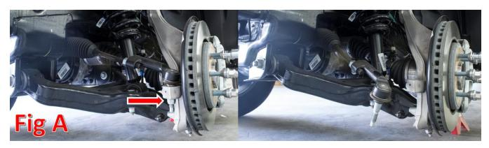
2. Loosen the OEM alignment nut, then use a crescent wrench to spin the OEM outer tie rod assembly off of the OEM inner tie rod end. Leave the alignment nut on the threaded post of the inner tie rod. (Fig B)
