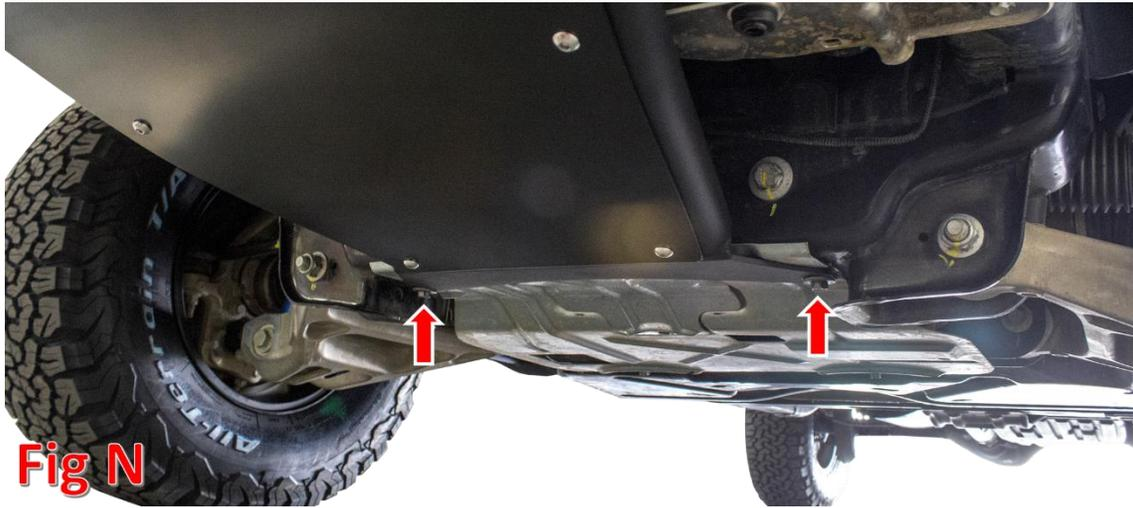
7. Align the bumper so that it is straight in relation to the grill/headlight bezels. You may need one person to hold the bumper in place while another person tightens the bolts.
