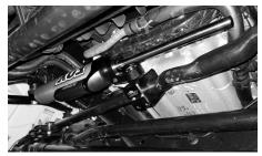
Fig. 2: Stabilizer clamped to drag link
